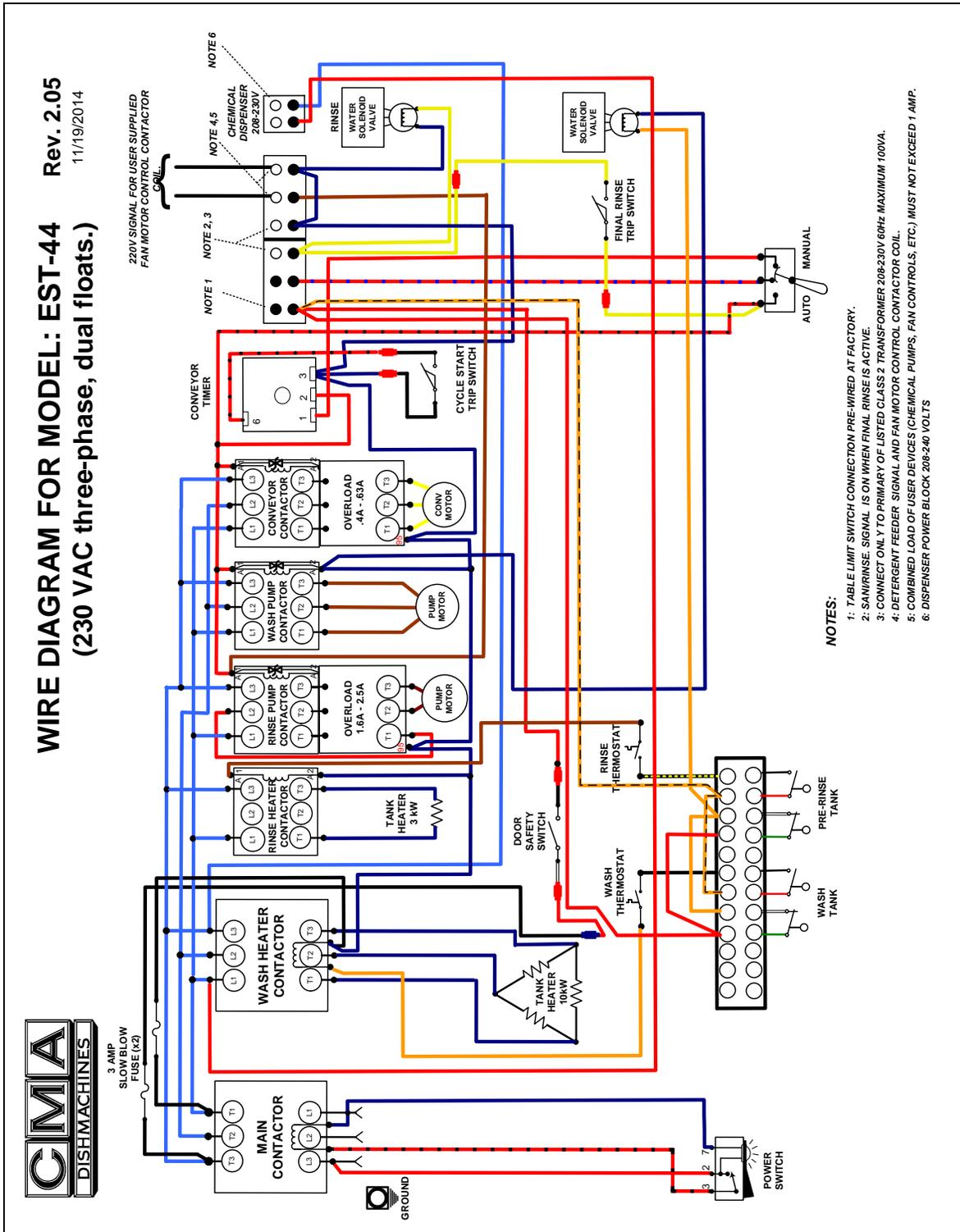
5. Electrical Diagram For E-Temp Heater Only
